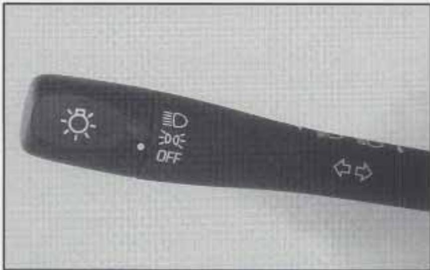
Rotate the turn signal lever end cap up one position to turn on:
