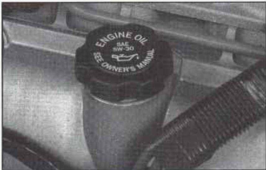
The oil fill cap for the 3100 engine is located on the front of the engine.
