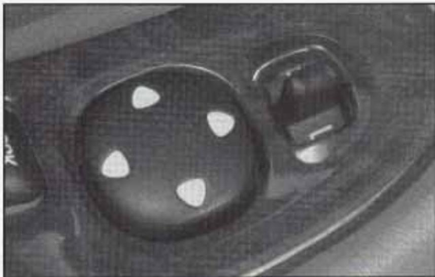
This switch is located on the armrest of the driver's door. Move this switch to the left or right depending on which mirror you need to adjust (center is the off position.) Then adjust the direction of the mirror using the paddle marked with arrows just below the selector switch.
