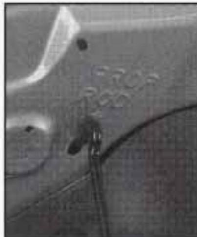
Lift the hood, release the hood prop from its retainer and put the hood prop into the slot marked PROP ROD.
