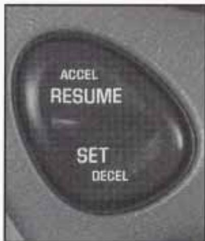
With cruise control, you can maintain a speed of about 25 mph (40 km/h) or more without keeping your foot on the accelerator. This can really help on long trips. Cruise control does not work at speeds below 25 mph (40 km/h).
