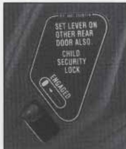
Your Oldsmobile is equipped with rear door security locks that help prevent passengers from opening the rear doors of your vehicle from the inside.
