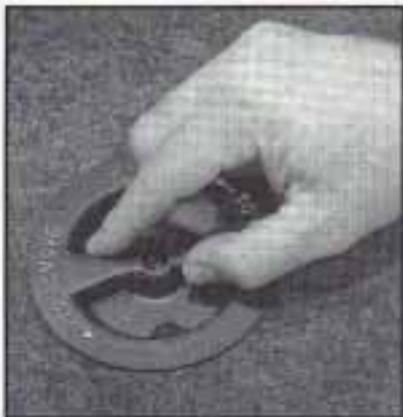
The equipment you'll need is in the trunk. Turn the center retainer nut on the compact spare cover to the left to remove it.
