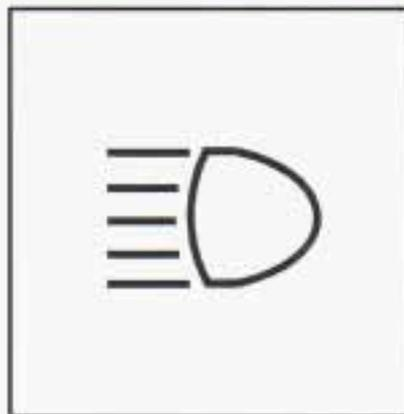
To change the headlamps from low beam to high beam, push forward on the turn signal/multifunction lever. To change the headlamps from high beam to low beam, pull the turn signal lever backward. When the high beams are on, a light on the instrument panel also will be on.
