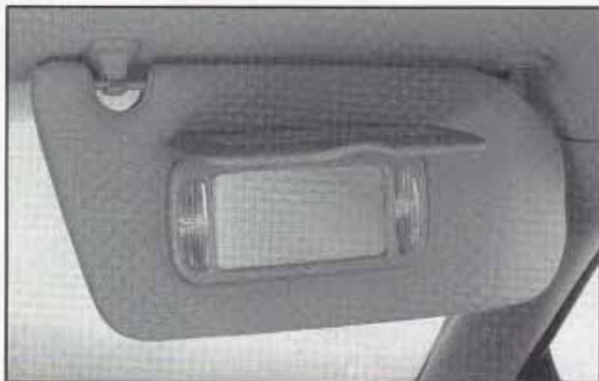
This mirror is located on the passenger's side visor. When you lift the cover, the light will turn on.
