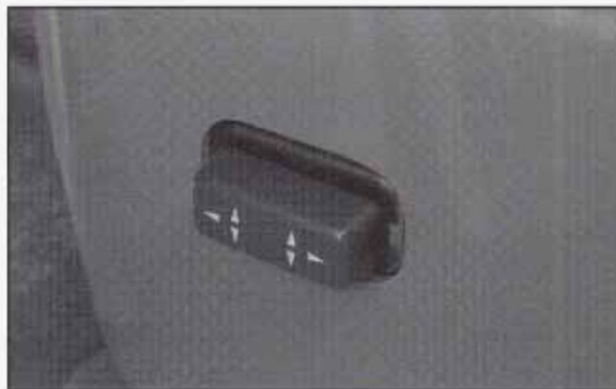
The power set button is located on the lower, left side of the driver's seat. This button allows you to move the seat up, down, forward and backward. It also moves the front of the seat up or down and the rear of the seat up or down.
