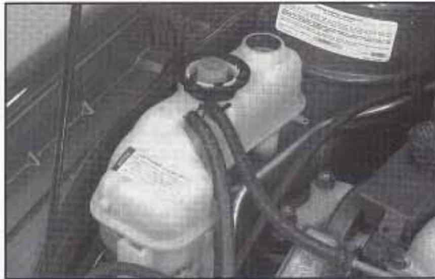
1. You can remove the coolant surge tank pressure cap when the cooling system, including the coolant surge tank pressure cap and upper radiator hose, is no longer hot. Turn the pressure cap slowly about one-quarter of a turn to the left and then stop.
