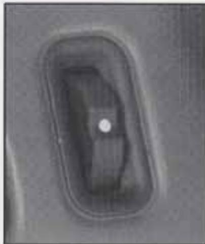
You can brighten or dim the instrument panel cluster lights by rotating the switch, located to the left of the steering wheel.
