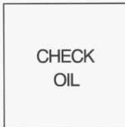
If the light comes on and you hear a chime or stays on after starting your vehicle, your engine oil level should be checked.
