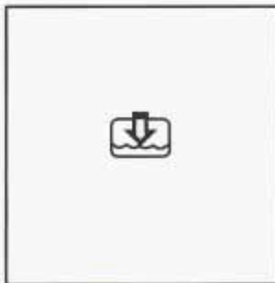
If the light comes on, it means you're low on engine coolant.
