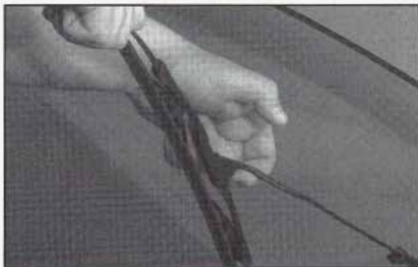
Replacement blades come in different types and are removed in different ways. For the proper type and length, see “Capacities and Specifications” in the Index. Here’s how to remove the Sheppard’s Hook type:
