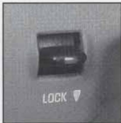
With the power door locks, you can unlock or lock all of the doors of your vehicle from the driver or front passenger door lock switch.
